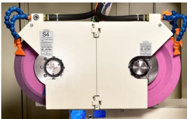
An example of an external and surface grinding unit with a straight (cylindrical) external grinding wheel as well as an external and surface grinding wheel profiled on both sides (alternating use via the round table - B3 axis)
