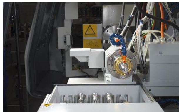
An example of a tool changer that is integrated into the machine which also allows the machining of workpieces and measurements
