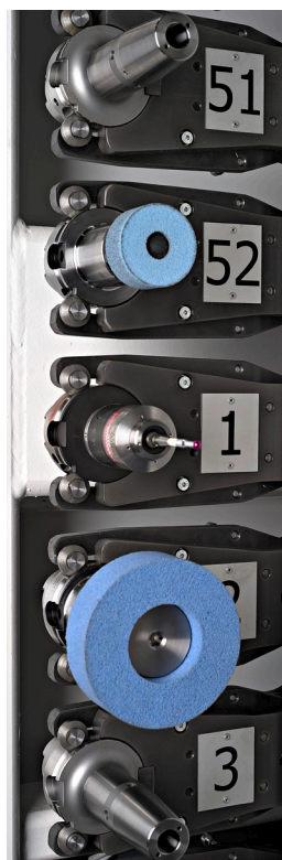
Example of a 52-position tool changer and the tool changing process for the complete machining of complex components in a single setup
