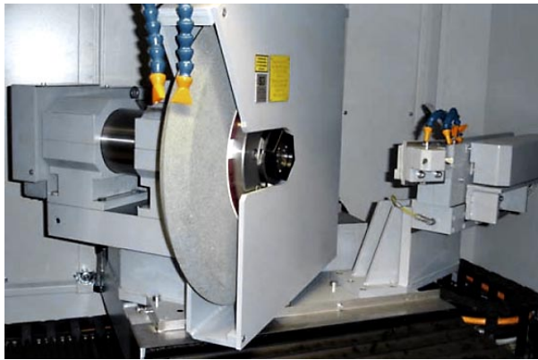
An example of an external and surface grinding unit at an angle of 45° in relation to the workpiece axis with external and surface grinding wheel profiled on both sides
